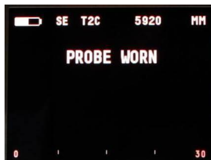
Probe Worn Message on Measurement Screen.
