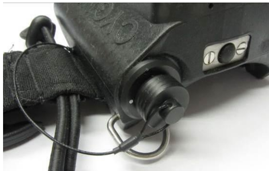
Probe Socket Cap Correctly Fitted.
