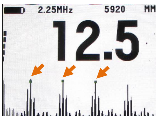
Flat, new steel 12.5mm thick.
