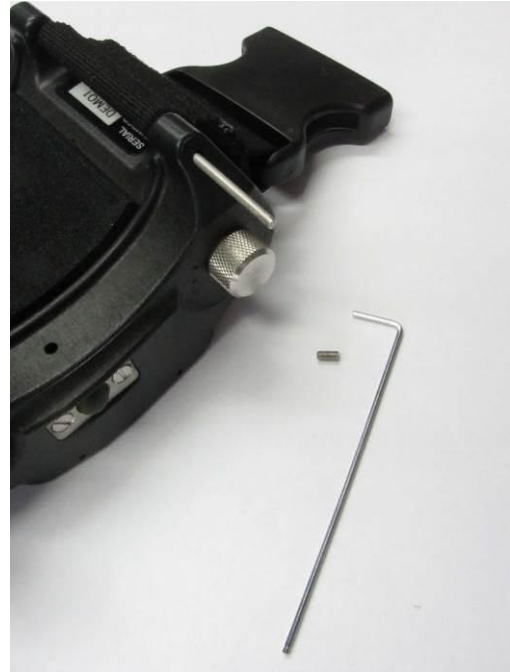
Wrist Strap Pin Securing Grub Screw
