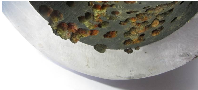
Large Corrosion Pits.
