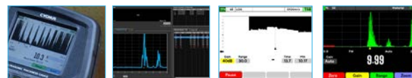
LARGE 3.5" OUTDOOR READABLE DISPLAY CYMLINK SOFTWARE B-SCAN WITH AUTO START/ PAUSE/CONTINUE LIVE A-SCAN FOR FURTHER VERIFICATION
