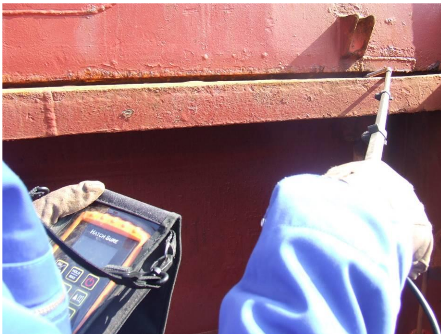
Fig 7.7. Pinpointing a Leaky Seal.
