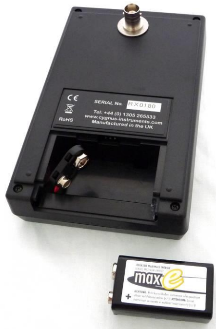
Fig 4.3 Receiver Battery Location
