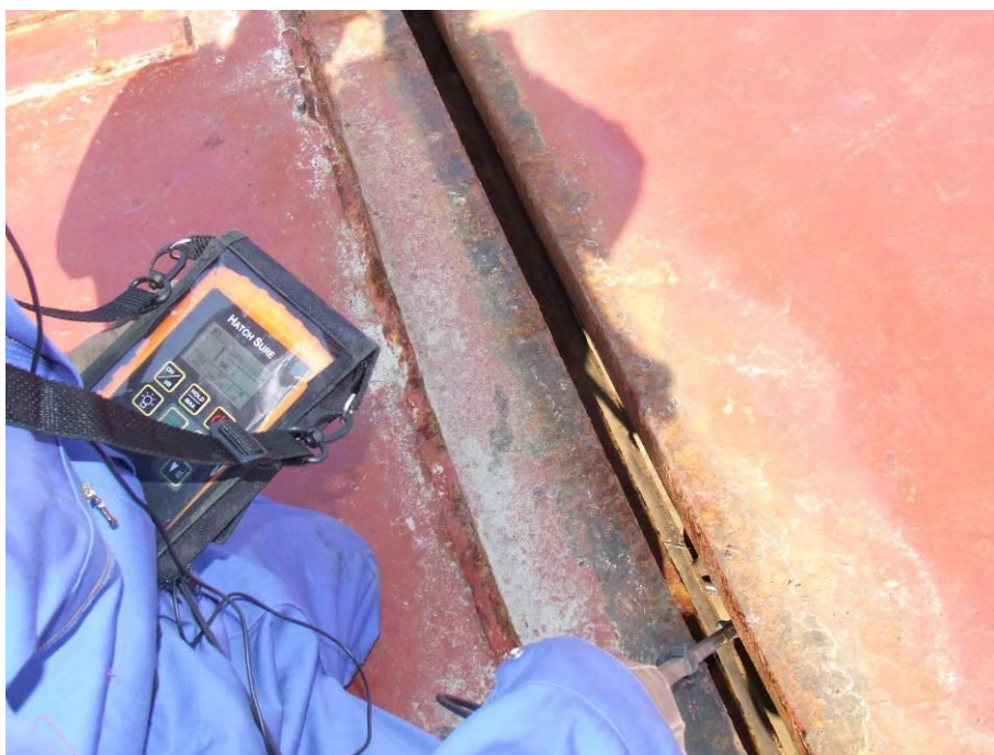
Fig 7.8. Scanning a Deep Hinged Joint.
