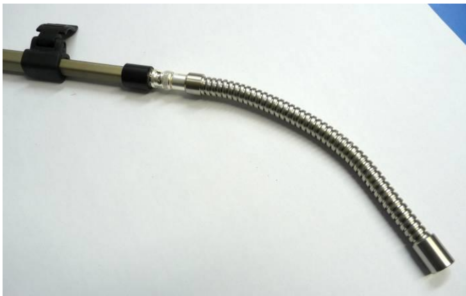
Fig 5.2 Inspection Microphone Connected to the Telescopic Extension
