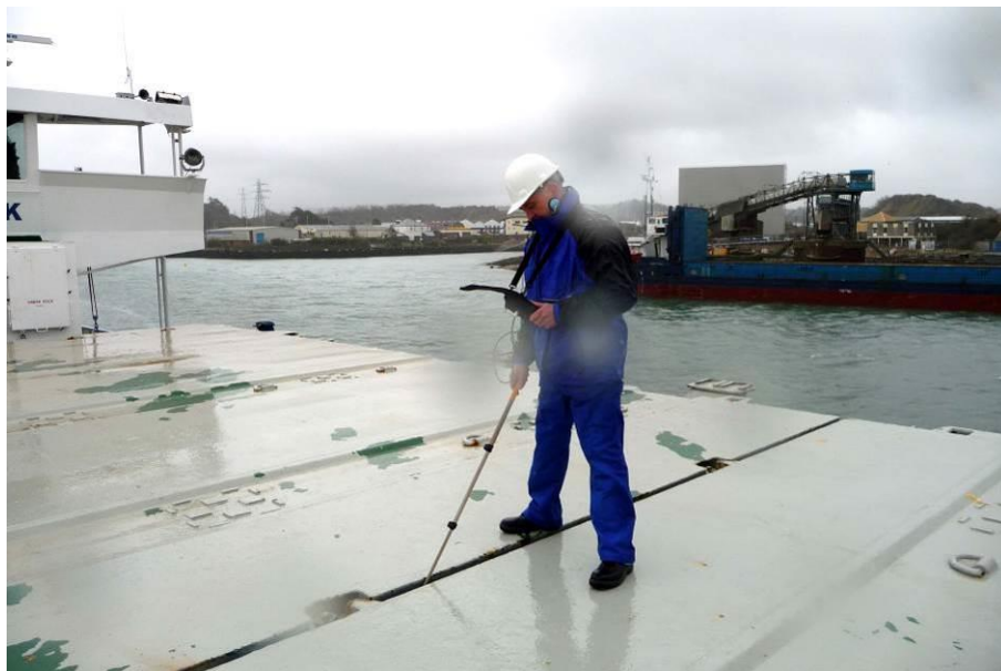
Fig 7.6. Scanning a Hatch Cover Joint.
