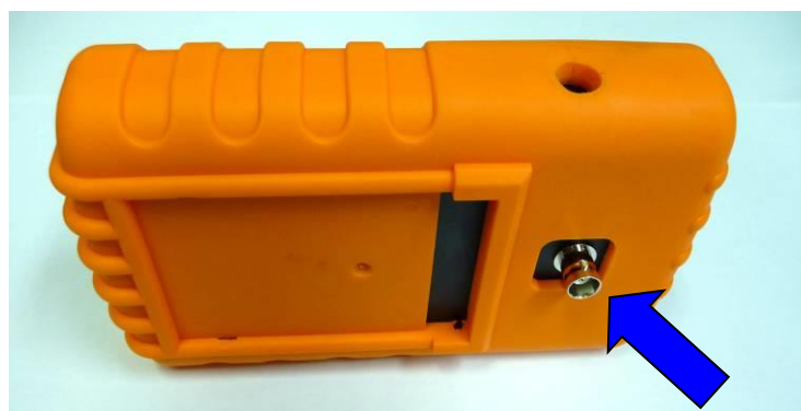
Fig 4.1 BNC Connection for Microphone
