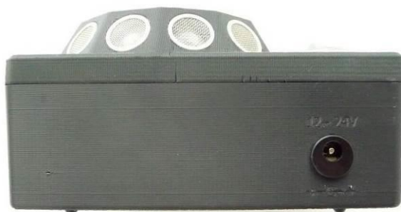
Fig 3.4 External 12-24 V dc Power Input
