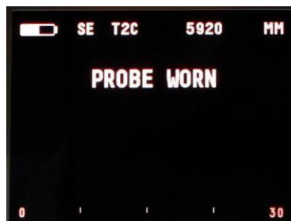
Probe Worn Message on Measurement Screen.
