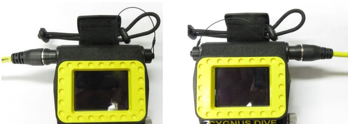
Right and Left Handed Probe Connections
