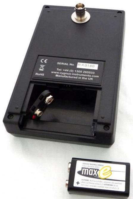
Fig 4.3 Receiver Battery Location
