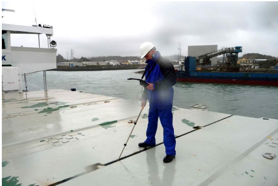
Fig 7.6. Scanning a Hatch Cover Joint.
