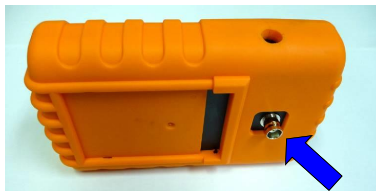
Fig 4.1 BNC Connection for Microphone
