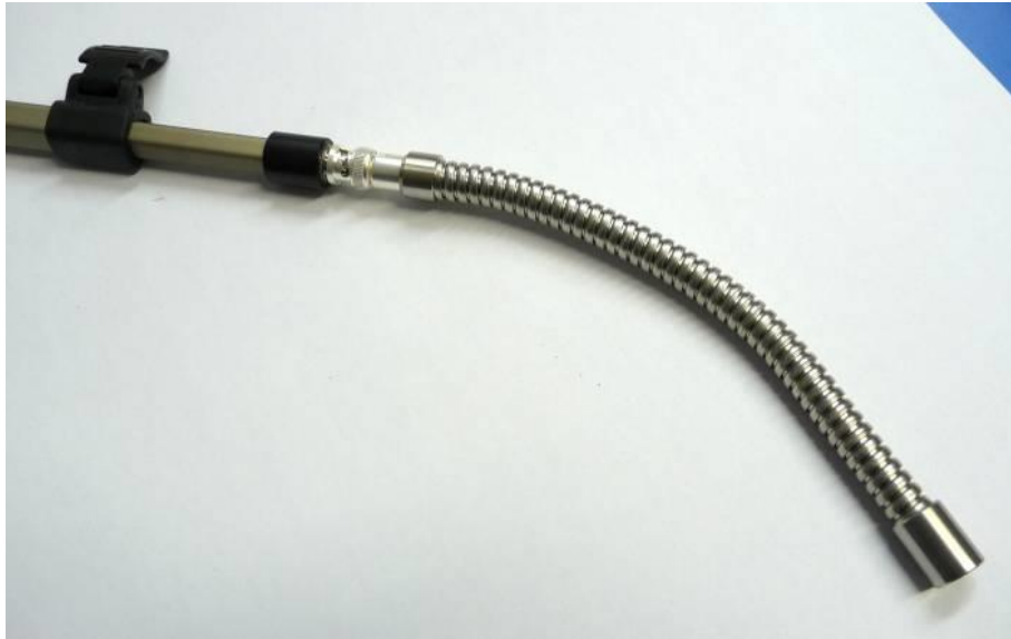
Fig 5.2 Inspection Microphone Connected to the Telescopic Extension
