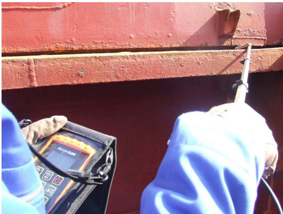
Fig 7.7. Pinpointing a Leaky Seal.
