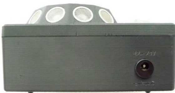
Fig 3.4 External 12-24 V dc Power Input
