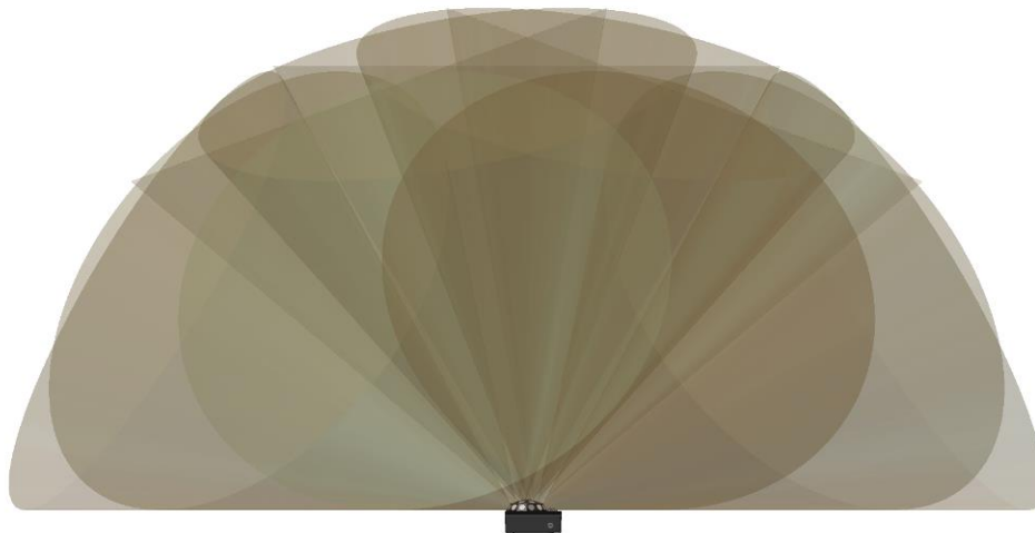
Fig 7.0a Transmitter Beam Spread Pattern (side view)
