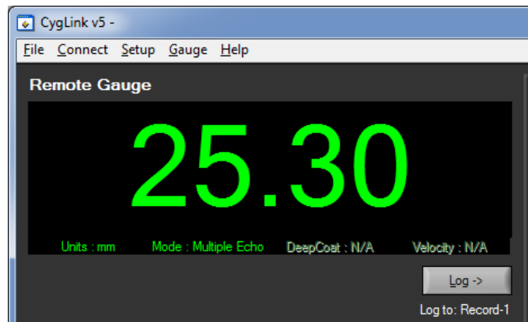
Topside Thickness Measurement and Log Button.
