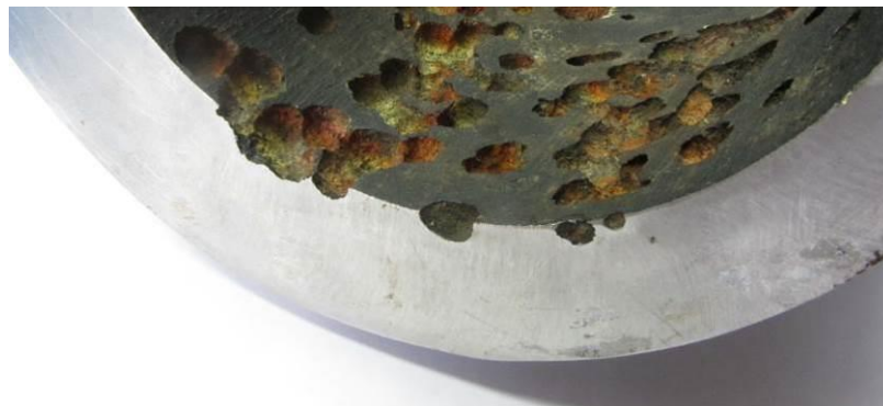
Large Corrosion Pits.
