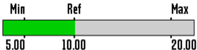
Thickness Measurement = Reference = Light Green Bar.
